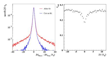
**Fig. 2.** Left: resolution on  $\Delta \tau$  variable evaluated from MC simulation as the difference between true values and data-like reconstructed values. The effect of the cut on the opening angle between tracks is shown. Right: total detection efficiency as a function of true  $\Delta \tau$  as observed from MC simulation. The dip around  $\Delta \tau \sim 0$  is discussed in the text.
